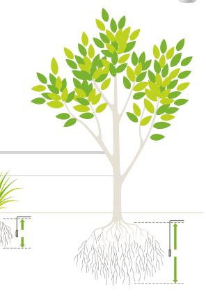
In turf applications, the probe should be placed in the root zone, approximately 15 cm deep (adjust for actual turf conditions).
